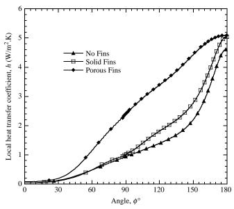
**Figure 5.**Distribution of heat transfer coefficients at the outer cylinder
